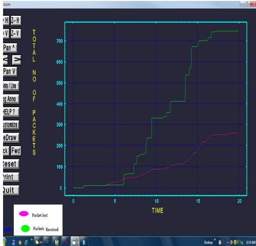
Fig. 3.5 Total no of packets received and lost in DSDV Protocol using 50 nodes network scenario.
