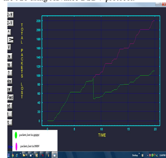
Fig. 4.4 Total no of packets lost in DSDV and Advance DSDV Protocol using 25 nodes network scenario.
