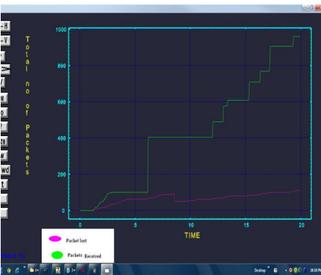
Fig. 3.2 Total no of packets received and lost in Advance DSDV Protocol using 25 nodes network scenario.
