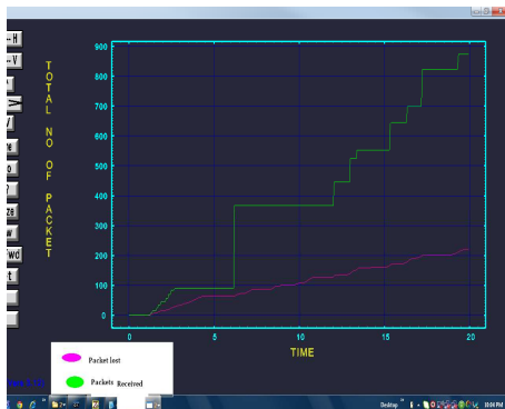
Fig. 3.1 Total no of packets received and lost in DSDV Protocol using 25 nodes network scenario.
