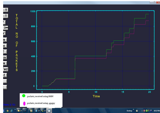
Fig. 3.3 Total no of packets received in DSDV and Advance Protocol using 25 nodes network scenario.
